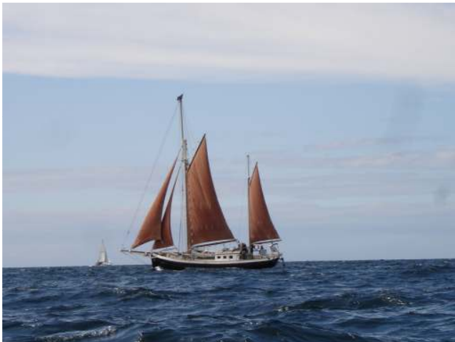
Cutter-headed Gaff Ketch, seen at Peel Traditional Boat Weekend 2013. Editor's own photo.
