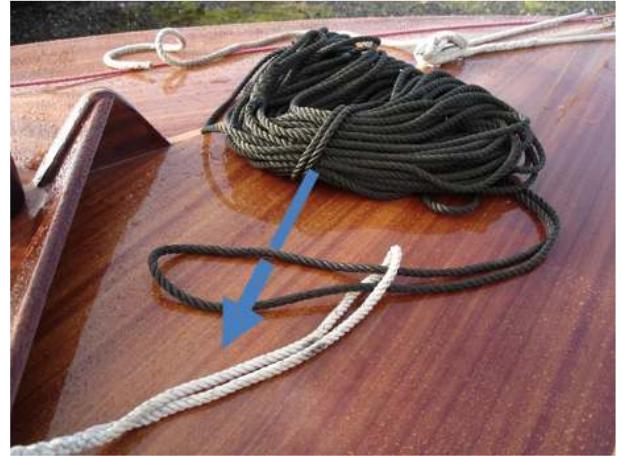
Long eyesplice on extension passed through eyesplice in bitter end of anchor warp. Skein will then go through the emerging loop, as shown by arrow.
