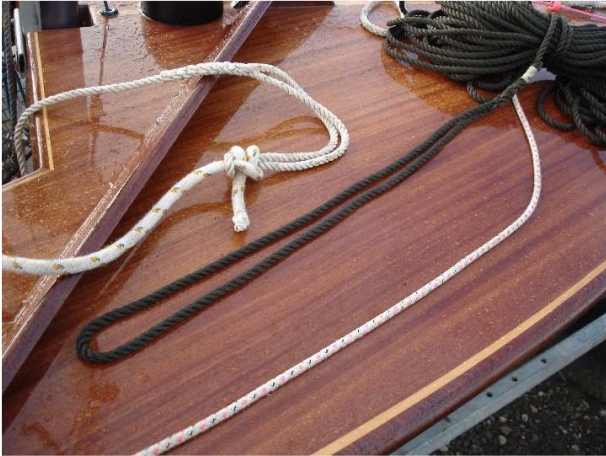
Eyesplice in bitter end of anchor warp tied to fixed rope, which is untied if ever I need to extend the warp. Also showing very long soft eye in extension warp
